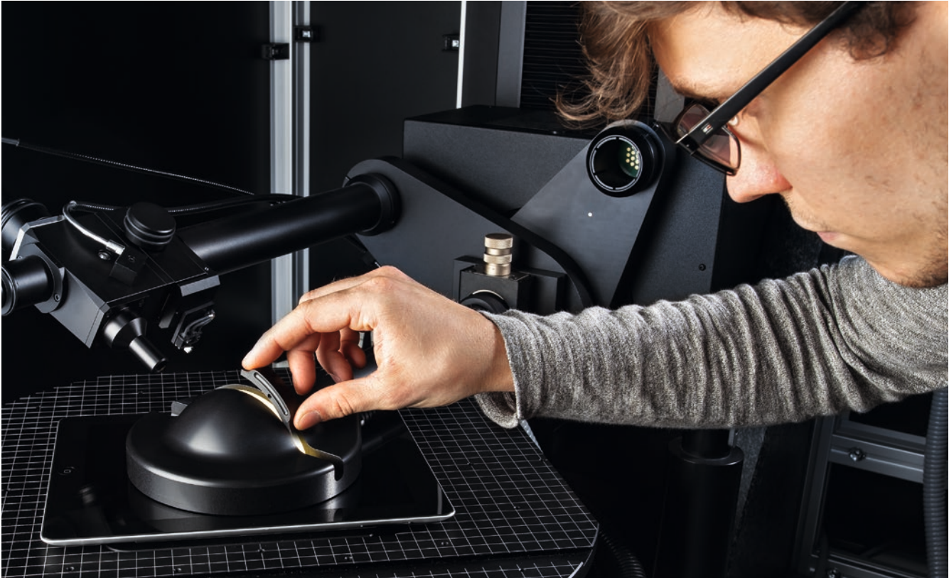
Fig. 1: The diffusing hemisphere is a valuable DMS-accessory for contrast measurement of reflective displays
