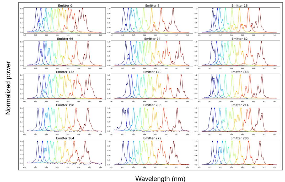
We have chosen 15 emitters at different locations across the array to perform spectrum analysis. The spectrum of these emitters are measured at different currents. Each subplot is an emitter with its spectrum at different currents (blue at 400 mA up to red at 1.8 A). We observe that there is a spectrum shift at higher currents and as well high order modes appear by current increase.
