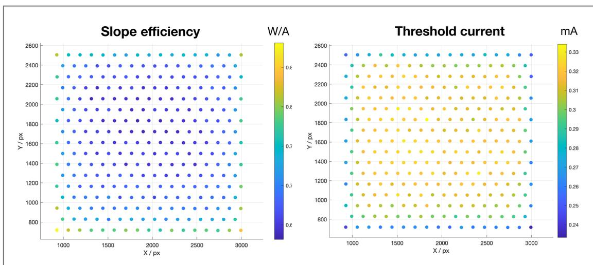
The slope efficiency and the threshold current of each individual emitter of the array was measured. The outer emitters have higher slope efficiency but lower threshold current.
